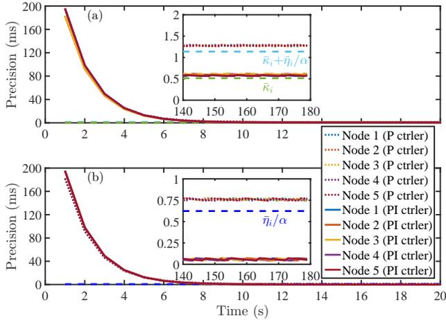
Fig. 6. Evolution of the synchronisation precision under the P-based and PI-based PkCOs algorithms.
