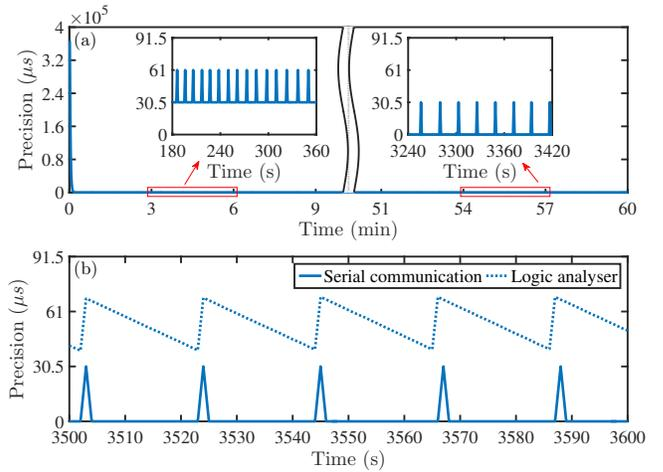
Fig. 10. Long-term stability of the PI-based PkCOs scheme.
